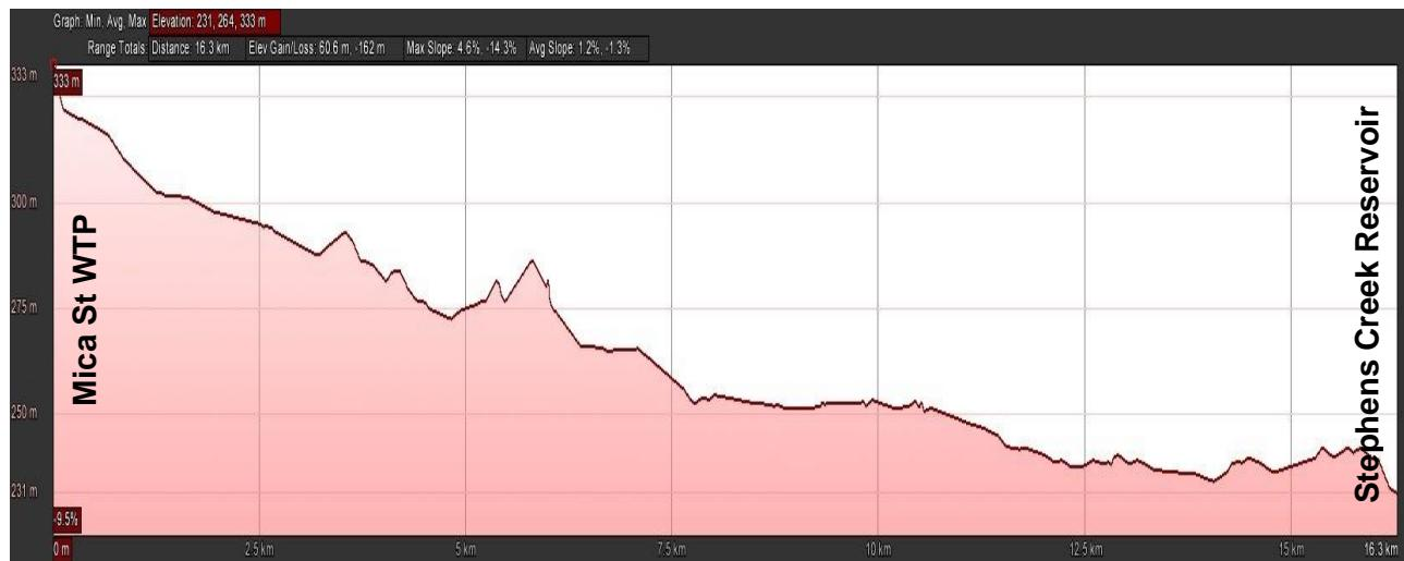
**Figure 3-3: Long-section profile of Stephens Creek Reservoir to Mica St WTP**
