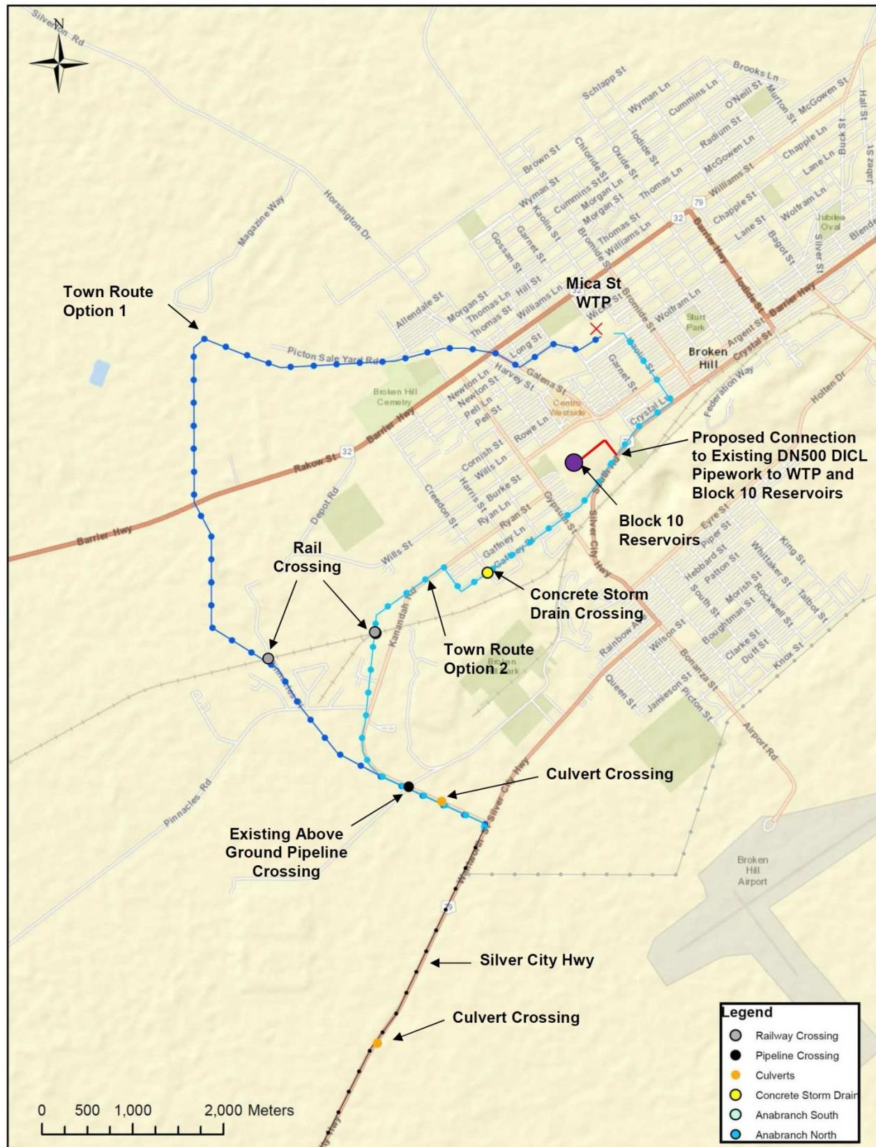
Figure 2-5: Plan of general overall route with topography DEM overlay
